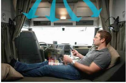
Park Cooler equipment, being independent from the engine, allows great fuel savings, avoids unnecessary use of the engine at idle and therefore a decrease in engine wear. If one takes into account that a truck consumes between 4 and 7 liters per hour at idle; depending on the type of the truck and the use, the equipment can be amortized in less than 4 months, just by saving fuel regardless of engine wear.
